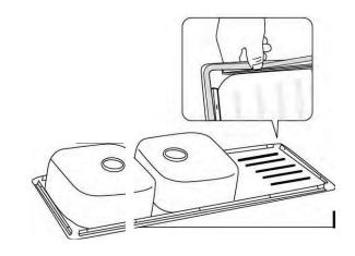
Adhere the seal tape around the under side of the edge of the sink, being careful to lay it smoothly (without ridges).
