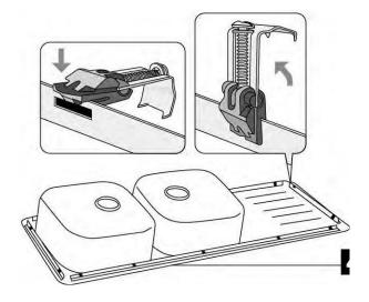
Place the anchor braces vertically and pull them up to lock into their horizontal position.
