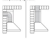
Maximum ducting distance should be 3 meters, with one 90 degree bend. For each additional 90 degree bend, the maximum distance is reduced by 1 meter. If the ducting is not correct it will increase noise and reduce performance.
