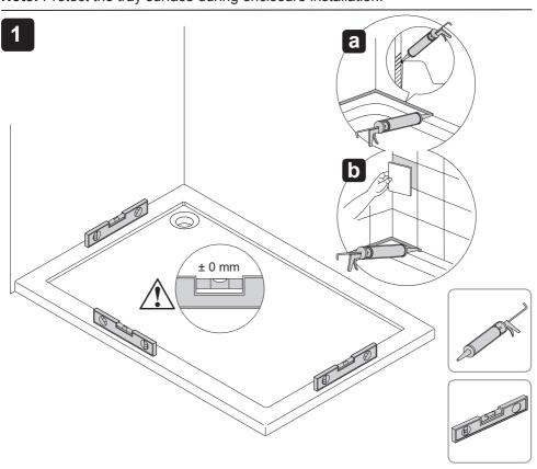
**Note!** Make sure that the walls have been tiled down to the tray. Make sure the Tray is levelled. Make sure the walls are flat and square.
