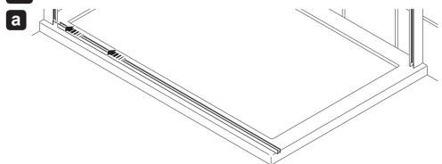
Note! Position the track so that the black gasket is on the fixed panel side for the glass to rest on and that the locating blocks are on the open door side.
