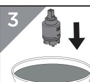
Place cartridge in a suitable solution and soak until fully de-scaled.
