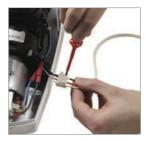
Prior to refitting the front cover, temporarily refit the temperature lever and rotate to the mid blend position (12 o'clock). Remove the lever and refit the front cover by locating the bottom of the front cover into the fixing lugs and pushing the front cover fully home. Secure using the fixing screw at the top of the front cover ensuring not to overtighten.
